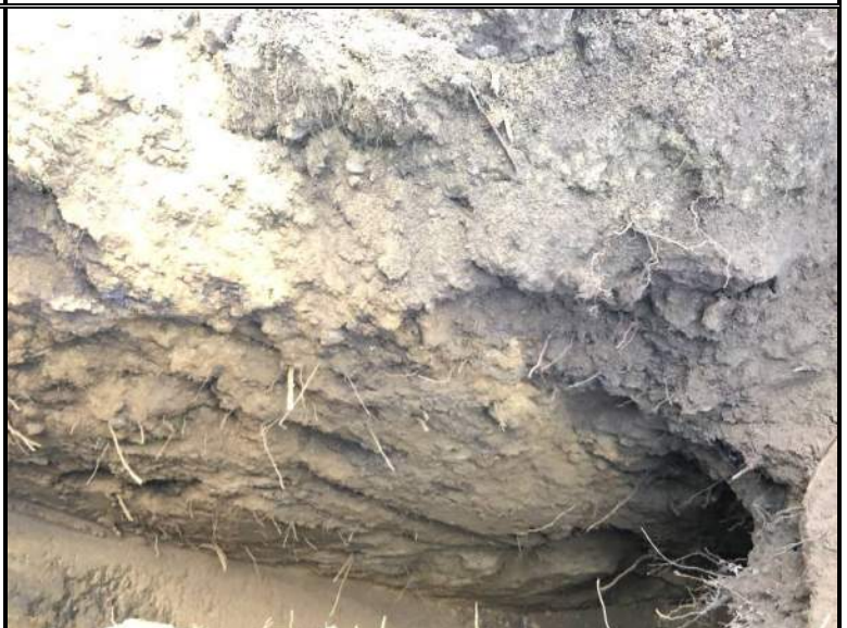
Exposed subsurface soil profile within test-pit TP-10
