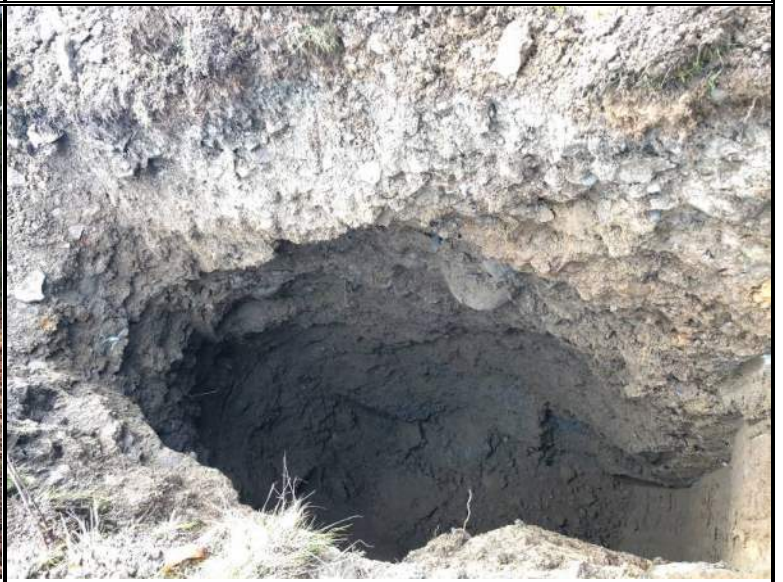
Exposed subsurface soil profile within test-pit TP-3
